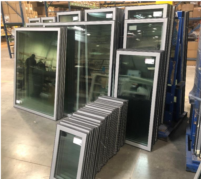
WinSert high performance window inserts for the VA building, manufactured in Colorado.
